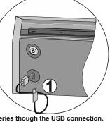
You cannot charge the safe's batteries though the USB connection.
