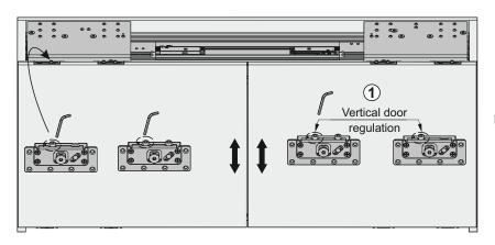
Regulate door position top-bottom with mounting plates' screws (1)
