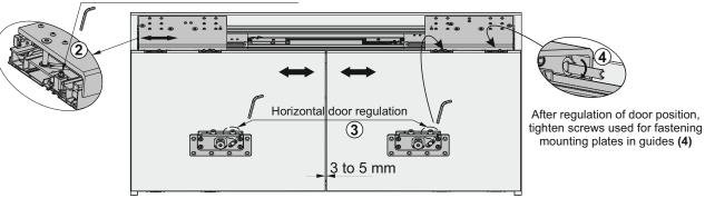
Regulate door position right-left with screws in mounting plates (3)
