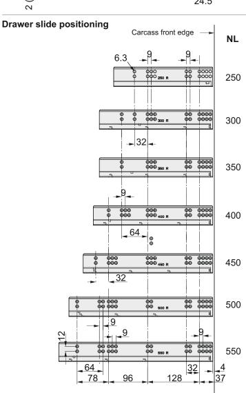
NL - nominal length of slide LT - internal cabin depth Drawer side thickness: 18 mm
