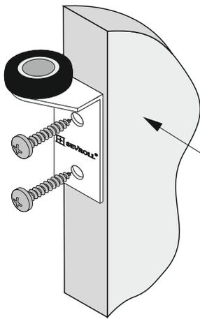
distancing guides should be fixed at a half way point of door height
