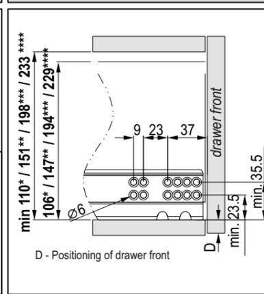
Mounting dimensions for drawer front panel
