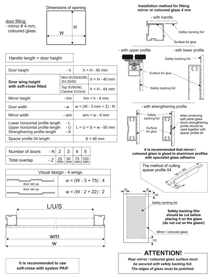
ATTENTION! Remove protective film from aluminium elements (handles, tracks, connectors, etc.) prior to cutting them to the desired size. Film removal will reveal quality issues (eg. scratches)
