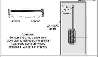
The Wardrobe lift can only be controlled by buttons, remote control, or voice commands. A power outage will prevent the wardrobe lift from operating.
