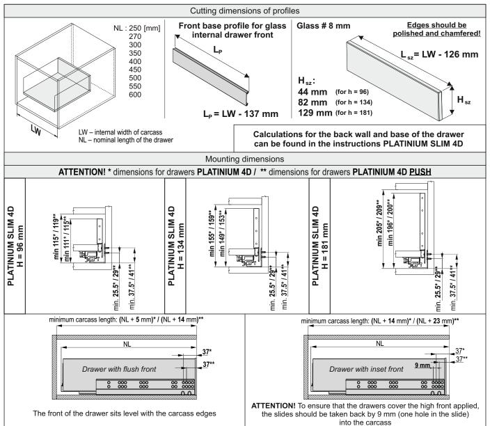
(If the drawer is fitted with LED lights, an additional space for activating the off switch must be taken into consideration)
