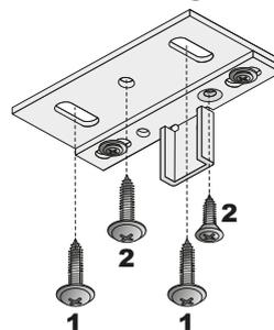
**1.** fix soft-close activator with screws 4x20.
