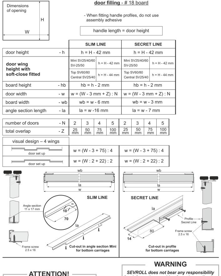
Handle profile should be 2 mm longer than board height. SEVROLL does not bear any responsibility for deformation resulting from the application of improper quality of boards (improper storage, improper humidity)
