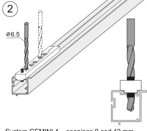
System GEMINI 4 – openings 9 and 42 mm System EDEN 4 – openings 21 and 55 mm
