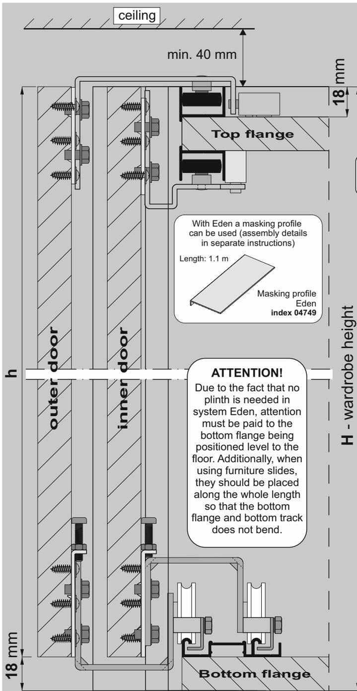
With Eden a masking profile can be used (assembly details in separate instructions)
