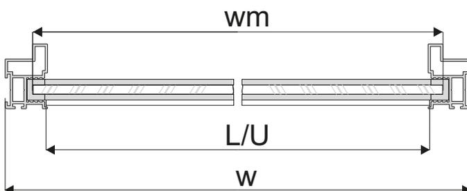
Installation method for fitting 10 mm board (diag. A) and 4 mm mirror or glass (diag. B)
