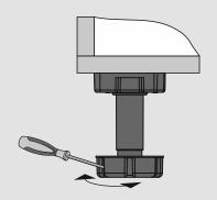
Adjustment with a screwdriver from front
