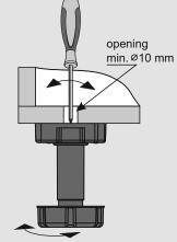
Adjustment with a screwdriver from above (be sure to use an appropriate screwdriver)
