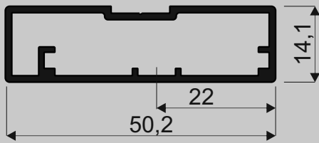
Strengthening profile S01, S02, S04, S05 (14x50 mm)
