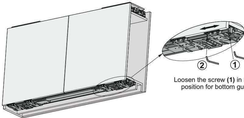
Loosen the screw (1) in bottom track, set optimal position for bottom guide (2), lock the screw
