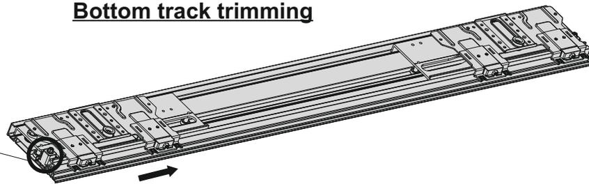
① Loosen the screw then shift the sliding mechanism right
