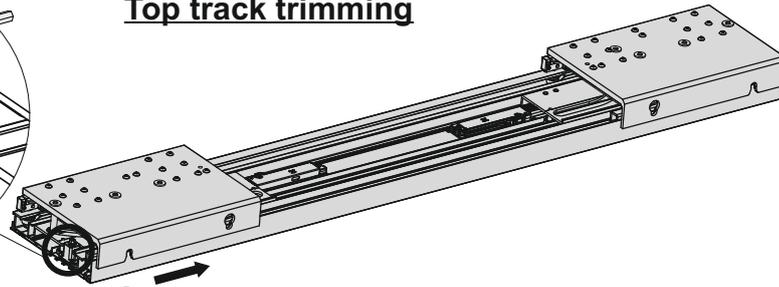
① Loosen the screw then shift the sliding mechanism right
