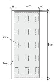
Broken line indicates recommended positioning od double-sided tape
