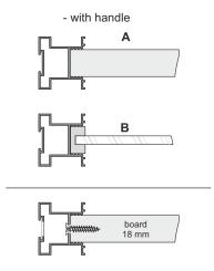
When using board, you can insert a screw (4x30) at mid-handle height for additional strength (in the same way as Maxim 18 Board system).
