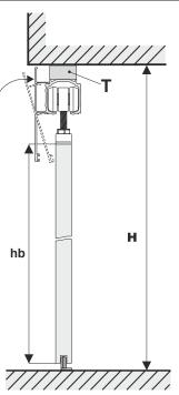
Top fastening of HERAKLES track - max. weight of 80 kg, 120 kg per door
