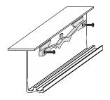
use self-tapping screw  $\varnothing 3.5$ or drill opening in track  $\varnothing 2.5$ and use Unix screw  $\varnothing 3.5$
