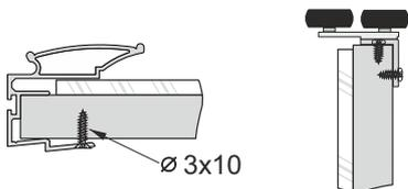
If the board or mirror is too loose on the handle profiles, screw the handles to the board using  $\text{Ø}3 \times 10$  screws.
