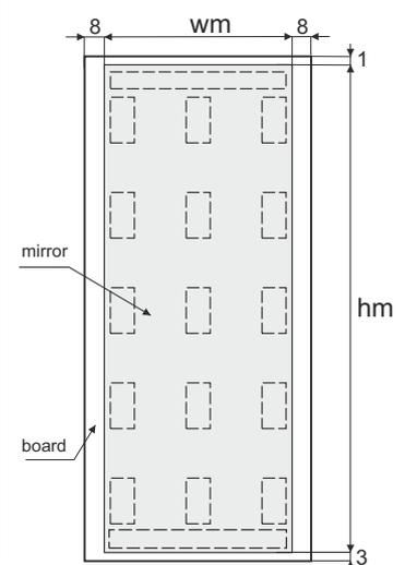
Broken line indicates recommended positioning of double-sided tape
