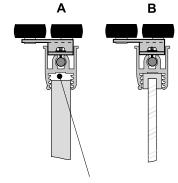
construction clearance included in the calculation of the height of board
