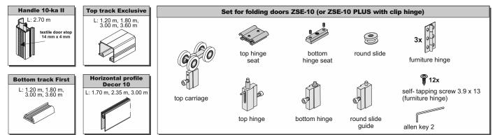
You must remember to purchase self-tapping screws 6.3x32 to construct each door (4 screws per door). When using safety glass or mirror, you must also remember to purchase gaskets.
