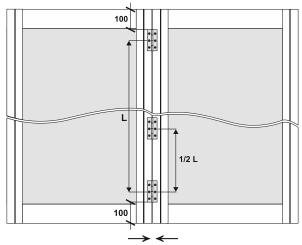
When fixing hinges, doors should be touching one another. Do not use textile door stop in between the touching handles!
