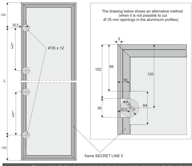
Method for positioning hinge recesses
