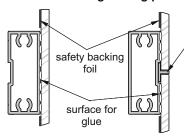
when producing split panel glass doors strengthening profile should be used together with spacer profile 04
