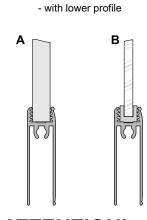
**ATTENTION!** Mirror (4 mm) should be used with a safety backing film. Safety glass (4.5 mm) comprises of two thin layers with a film in-between. Both mirror and glass need fitting gaskets.
