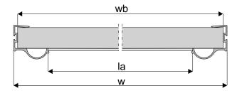
Handle profile should be 2 mm longer than board height.
