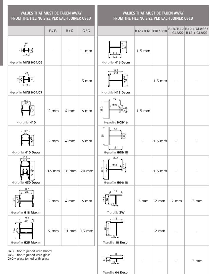
**B16/B16** – 16 mm board joined with 16 mm board **B18/B18** – 18 mm board joined with 18 mm board **B18/B12 + glass** – 18 mm board joined with 12 mm board and glass **B12 + glass/B12 + glass** – 12 mm board and glass joined with 12 mm board and glass
