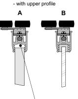
construction clearance included in the calculation of the height of board
