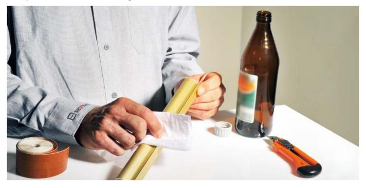
2 Apply foil by pressing the cloth into the handle
