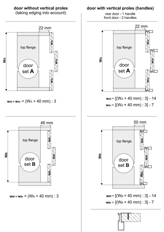
handle to be fastened with a minimum of 4 screws
