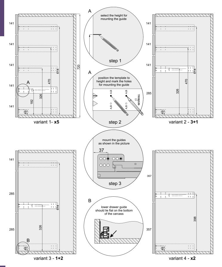
Marking holes for attaching the guides to Sevrollbox Slim drawers with **overlays** fronts
