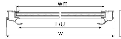
Installation method for fitting 10 mm board (diag. A) and 4 mm mirror or glass (diag. B)
