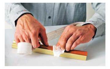
3 After application, cut off excess foil with retractable knife
