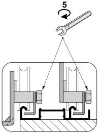
securing catch - fasten after door assembly
