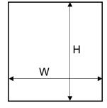
door filling: # 10 mm board, # 4 mm mirror or # 4.5 mm safety glass
