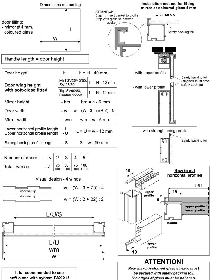
Remove protective film from aluminium elements (handles, tracks, connectors, etc.) prior to cutting them
