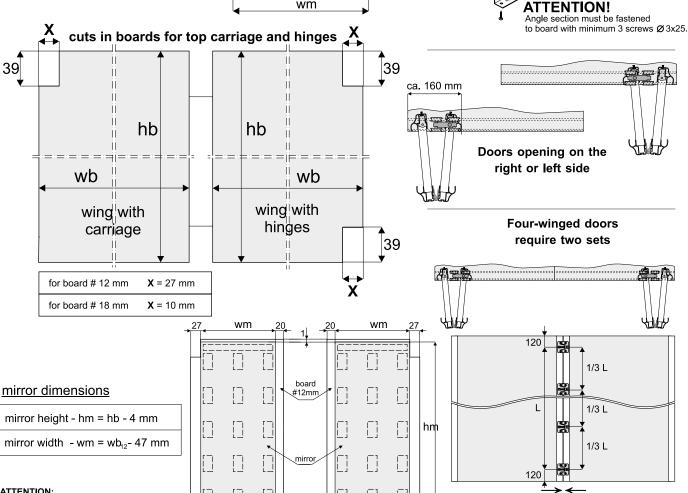
ATTENTION: Board to mirror contact area should be free from dirt and grease before applying double-sided tape..
