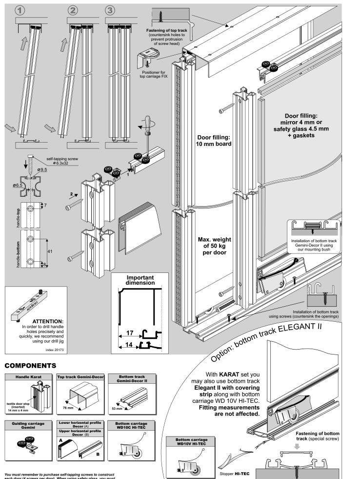
You must remember to purchase self-tapping screws to construct each door (4 screws per door). When using safety glass, you must also remember to purchase gaskets.
