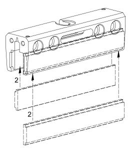
Installation of clamps on the glass 2 follow proper screws 1 tightening sequence 00 ~1kg **P** 00 1 F1 0 2 Ò 3 200-00 2 (1)(3) (4) F2 TIN T F2 > F1 ----~120 mm ~120 mm 4 A 00 00 (2) 3 1  $(\mathbf{4})$ F3 . F₃ ≈26 ̈́ Ņm (2) (3)  $(\mathbf{1})$  $(\mathbf{4})$
