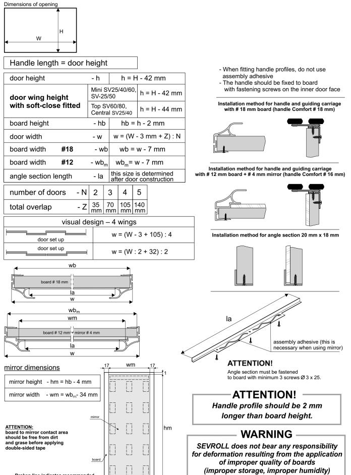
Broken line indicates recommended positioning of double-sided tape
