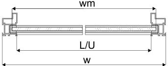
Installation method for fitting 10 mm board (diag. A) and 4 mm mirror or glass (diag. B)
