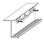
use self-tapping screw Ø3.5 or drill opening in track Ø2.5 and use Unix screw Ø3.5
