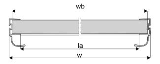
Handle profile should be 2 mm longer than board height.
