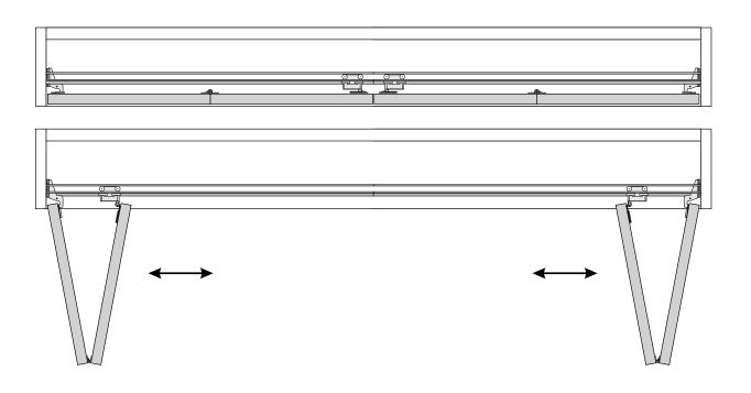
The assembly of folding doors **SLIM LINE** opened to the right and to the left side requires the use of two sets:
