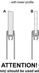
Mirror (4 mm) should be used with a safety backing film. Safety glass (4.5 mm) comprises of two thin layers with a film in-between. Both mirror and glass need fitting gaskets.
