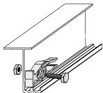
drill an opening in a track Ø 6
